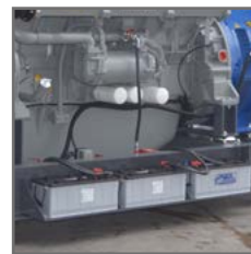
Battery holder designed to facilitate maintenance and replace
