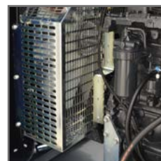
Rotating part guards to prevent injuries to the user
