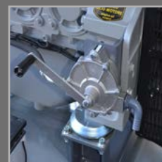
Oil change pump it facilitates oil change
